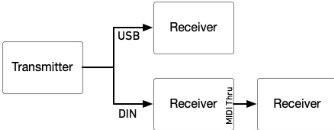
every quarter note (24 PPQ) and the receivers each calculate the tempo independently. Start, stop, and continue messages are used to synchronize playback between devices. The transmitter
