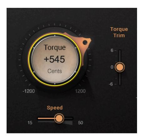
The **Torque Knob** controls the amount of formant shift. This action mostly affects the frequencies around the Focus setting. So if Torque is not correcting tone as expected, re-adjust the Focus setting.
