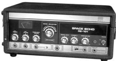
6•26 Long before Boss® pedals, the RE-101 Space Echo (which this model is based on\*) was Roland®'s first venture into the world of effects processing. Instead of having one movable playback head (like the Echoplex) this machine has multiple stationary heads. You change delay times by switching amongst these heads, and then fine-tune delay time with a motor speed control. The groovy part is that you can play back on multiple heads at the same time to get multi-tap delay effects.
