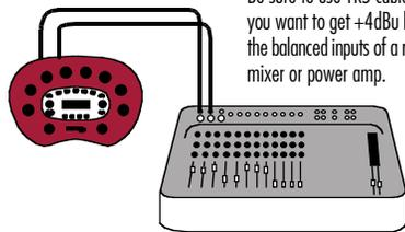
Be sure to use TRS cables when you want to get +4dBu levels to the balanced inputs of a recorder, mixer or power amp.
