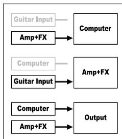
recording. As you can see from the diagram, the guitar goes right to the internal processing of the PODxt, the processed signal is sent to the computer (so you can record it) and the output of the PODxt shows both the processed guitar signal and the tracks that you're playing on the computer. Pretty straightforward, isn't it?
