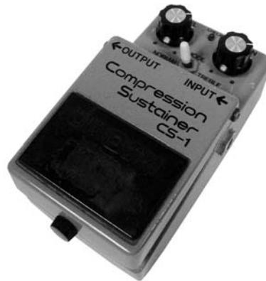
Roland®/Boss® jumped on the compressor stompbox bandwagon with the CS-1 Compression Sustainer. It has a fixed ratio, so the PODXT model based on\* it has the **SUSTAIN** control varying the threshold of the compressor circuitry. **LEVEL** does what you'd expect.
