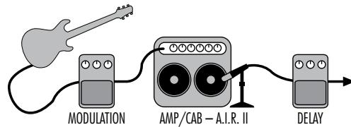
Here's another routing with both **MOD** and **DELAY** effects in the **PRE** position:
