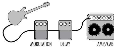
And this is what the full signal flow looks like inside your PODxt, including the pre and post options for Mod, Delay and the Volume pedal:
