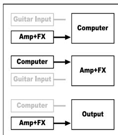
computer audio is sent to the internal processing of the PODxt, and the processed signal is fed back to the computer for recording and to the outputs of the PODxt for monitoring.
