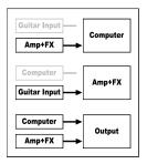
recording. As you can see from the diagram, the guitar goes right to the internal processing of the PODxt, the processed signal is sent to the computer (so you can record it) and the output of the PODxt shows both the processed guitar signal and the tracks that you're playing on the computer. Pretty straightforward, isn't it?
