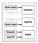
setting. The dry guitar input signal is sent to the computer for recording, and also to the internal processing of the PODxt so you can hear how the guitar sounds through the amp and effects you've dialed up. The tracks you're playing and the processed guitar signal are sent to the output of the PODxt so you can monitor your performance.
