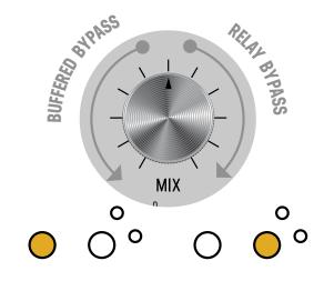
**(L)** LED indicates BUFFERED BYPASS
