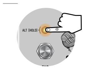
HOLD **(L)** LED switch on power up (power up takes 3 secs): all of the front panels LEDs will blink 3 times Power cycle to save setting
