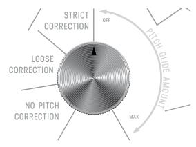
Hedra features 3 different pitch corrections settings or a pitch glide amount as listed in the knob graphic below. When Loose Correction is selected, the notes are forced into the current Key and Scale but pitch bending is not removed from the input. When Strict Correction is selected, the notes are forced into the current Key and Scale but pitch bending is removed from the input.
